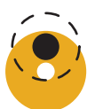
12mm badge with 3mm hole leaves just enough space for clutch pin
